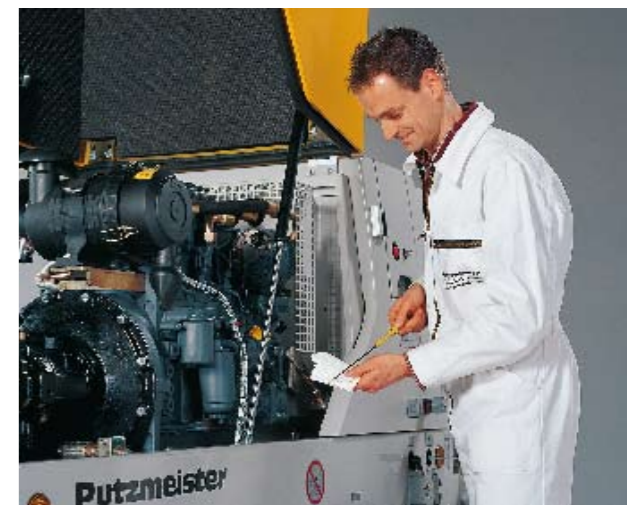
Nothing gets in the way. All the areas requiring service or maintenance are within convenient reach, as here, the oil level control.
