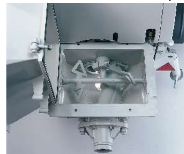
Just fold the hopper away to the side and the agitators are exposed and easily accessed.
